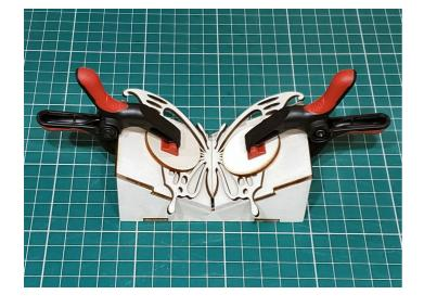
Apply a good-quality PVA wood glue, using the jig to ensure a precise 120-degree angle.
